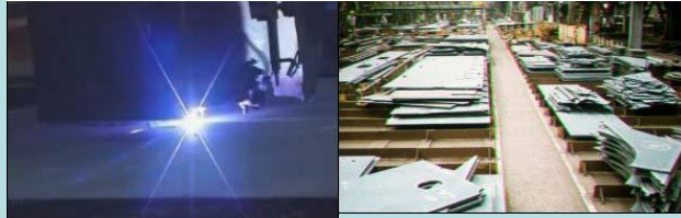
C. Steel cutting (S/C)
